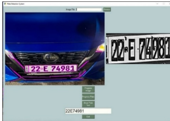
Figure 15. Final recognition result for ANPR system
